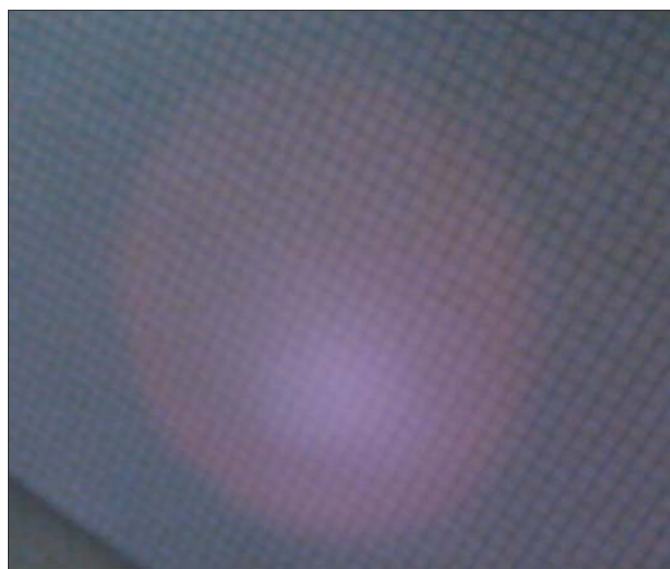
Figure 3. The aiming beam intensity of laser 6 complies with the IEC 60601 standard but the user does not have a correct information about the irradiated area
