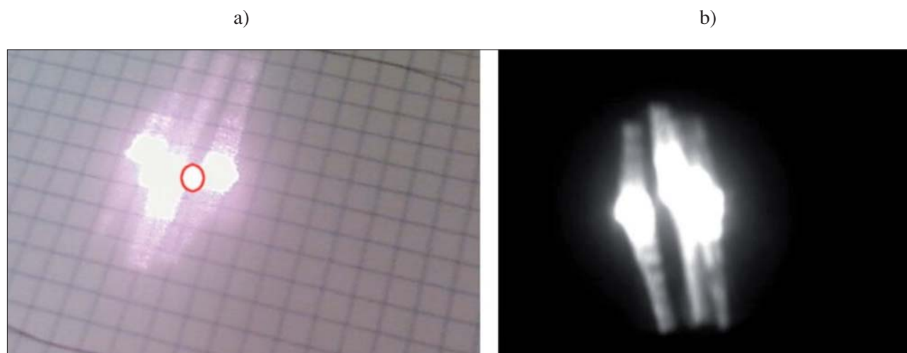
Figure 2. a) aiming beam (in the circle) and treatment beam are aligned but the treatment spot is not uniform, b) same laser spot captured by an IR camera
