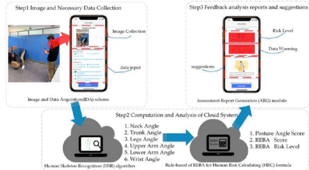
Figure 1. The system architecture of the Quick Capture system.
