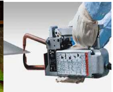
Welding manual resistance
