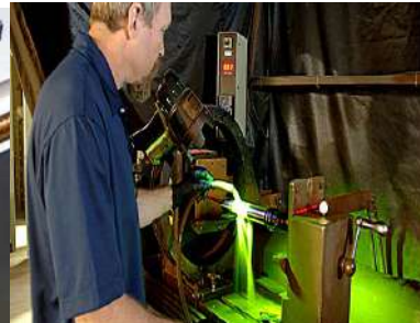
NDT Magnetic inspection
